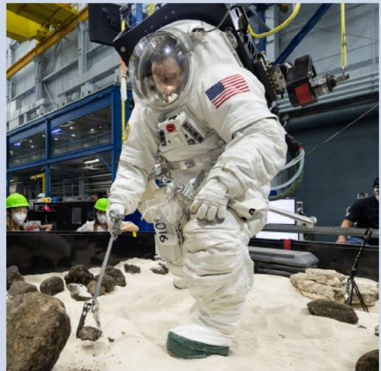
A NASA Engineer Uses Tongs to Pick Up Geology Samples During Testing at Johnson Space Center
