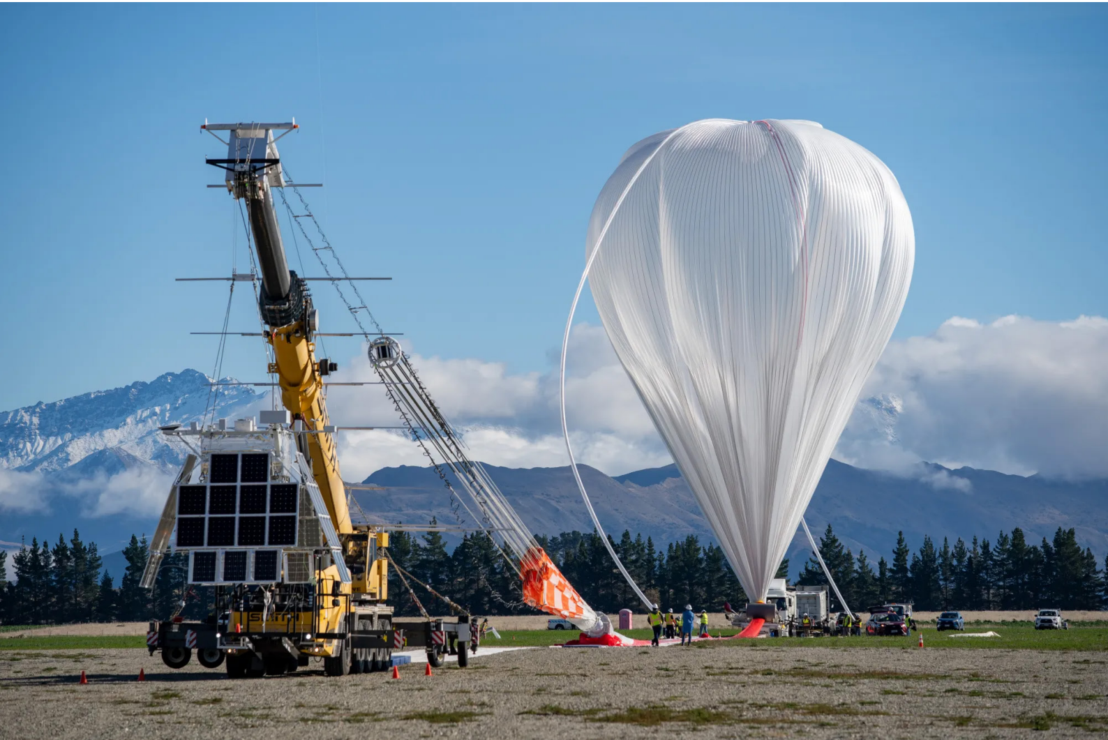
NASA's football-stadium-sized, heavy-lift super pressure balloon launched from New Zealand on May 3, 2025, to further test and qualify super pressure balloon technology.
