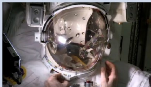
A water leak occurred in the helmet of Italian astronaut Luca Parmitano, forcing NASA to abort a July 16, 2013, spacewalk.
