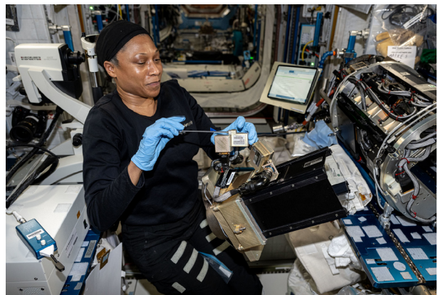
Aboard the ISS, NASA astronaut Jeanette Epps replaces and cleans research components inside the Combustion Integrated Rack, which is used for fire safety investigations.
