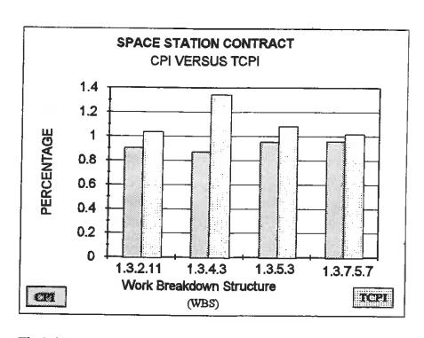
The TCPI represents what the contractor will have to achieve for the remaining work to stay within its current estimate at completion. In each of the WBSs selected, Boeing is projecting better performance for the remaining work than previously achieved.
