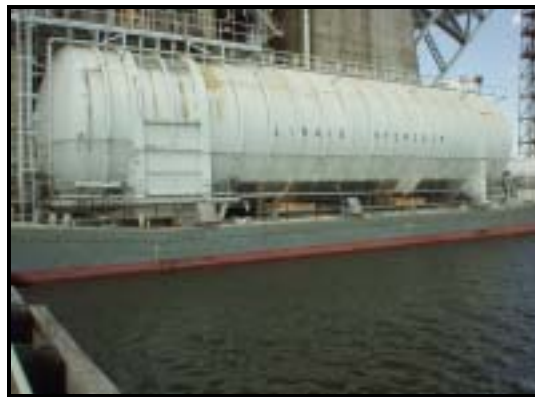
Figure 2. One of Stennis' three 270,000-gallon liquid hydrogen barges shown docked at the B1/B2 test facility.
