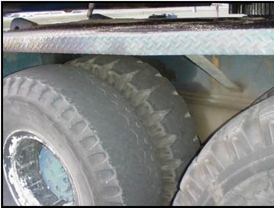
Figure-3. Bald tires on a 55-ton mobile crane.
