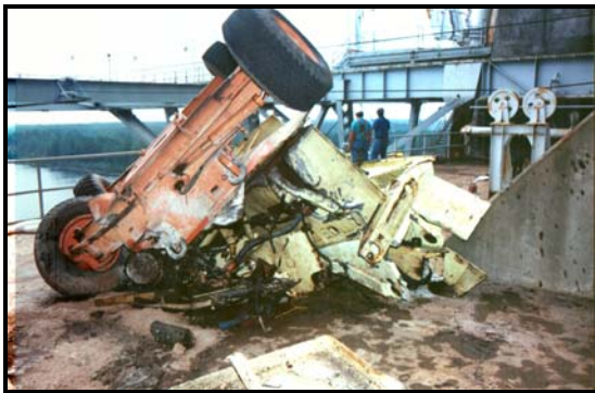
Figure 1. View of destroyed man-lift from the sixth level
