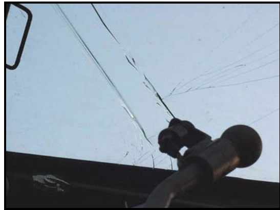
Figure-4. Cracked operator's cab roof glass on a 55-ton mobile crane.
