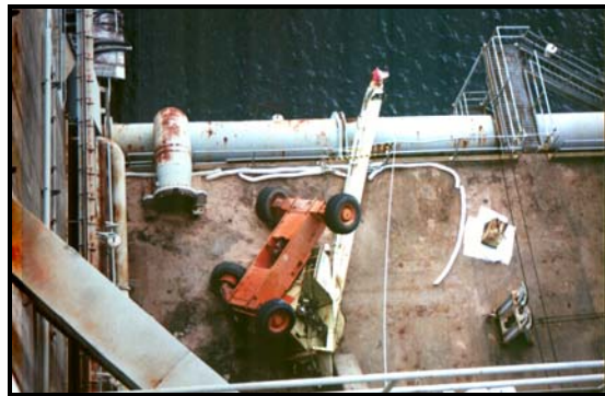
Figure 2. Overhead view of destroyed man-lift
