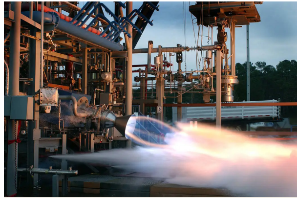
Next-generation pad abort demonstrator technology is tested by Boeing Rocketdyne at a test stand at NASA's Marshall Space Flight Center in Huntsville, Alabama.
