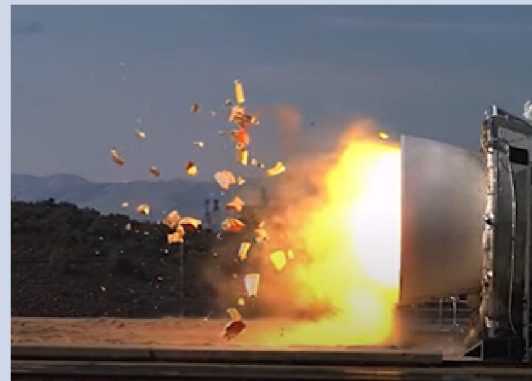
Throat plug debris shown liberating from the SLS booster nozzle during a 2016 ground test. The throat plug—designed to protect the booster before ignition—is rapidly expelled when the booster ignites.
