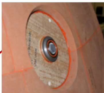
Figure 4: Orion Crew Module/Service Module Separation Bolt Melting and Erosion
