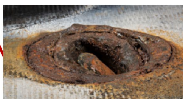
Separation bolt melting and erosion post-Artemis I reentry
