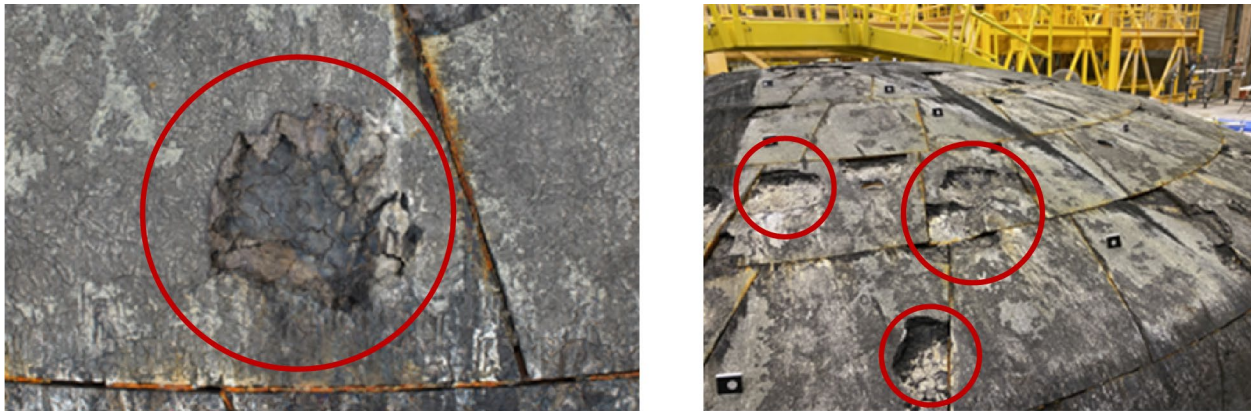
Figure 3: Orion Heat Shield Char Loss After Artemis I Mission
