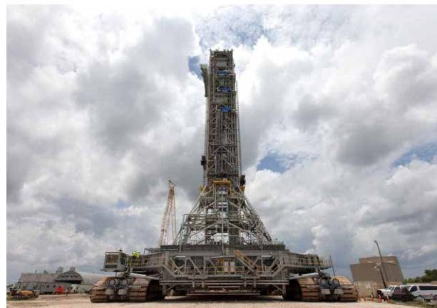
NASA's mobile launcher will assemble, process, and launch the SLS rocket
