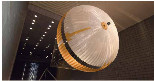
Mars parachute testing at Ames Research Center's National Full-Scale Aerodynamic Complex
