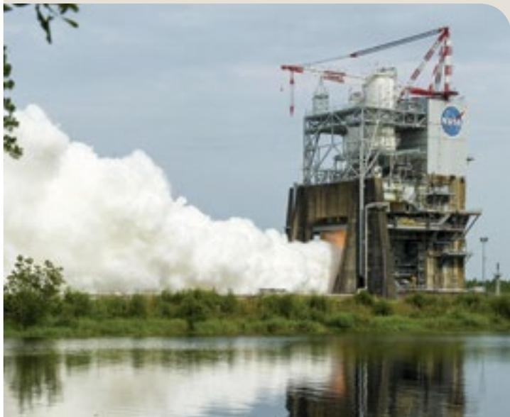
SLS rocket engine test at Stennis Space Center
