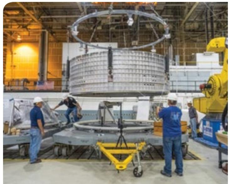
**Welding preparations for the Orion spacecraft at Michoud Assembly Facility**
