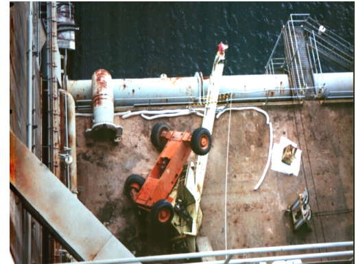
Overhead view of destroyed man-lift
