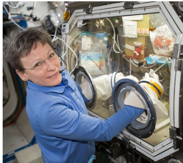
**Microgravity Science Glovebox inside the ISS National Laboratory**
