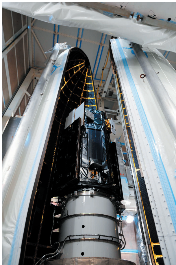
Encapsulation of NASA's Orbiting Carbon Observatory-2, or OCO-2, into the Delta II payload fairing nears completion in the mobile service tower at Space Launch Complex 2 on Vandenberg Air Force Base in California.
