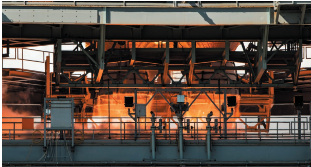
The four RS-25 engines on NASA's SLS rocket—as pictured above during the March 2021 SLS core stage Green Run hot fire test at Stennis Space Center—produce more than 2 million pounds of thrust.
