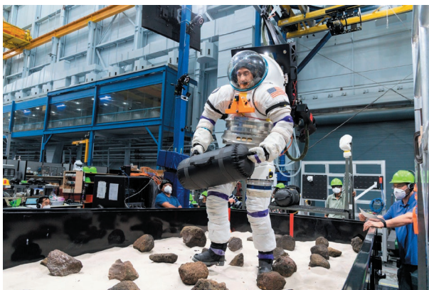
A volunteer from NASA’s Artemis Extravehicular Activity training group moves a 30-pound object through a boulder field while in a spacesuit connected to NASA’s Active Response Gravity Offload System.
