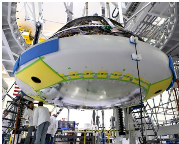
Engineers and technicians install the heat shield onto the Orion crew module
