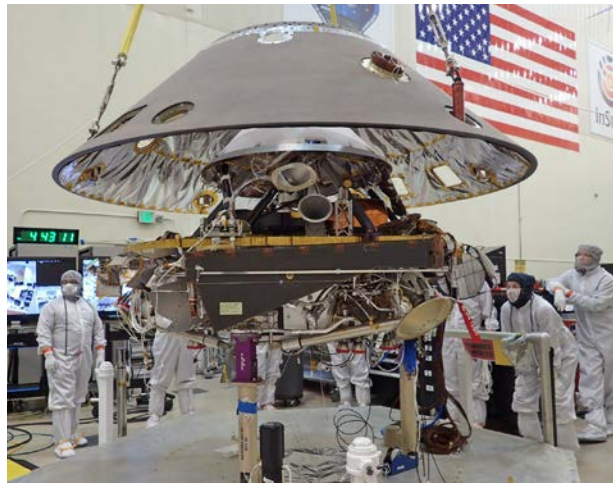
The back shell of the InSight spacecraft is lowered onto the lander in a clean room at Lockheed Martin
