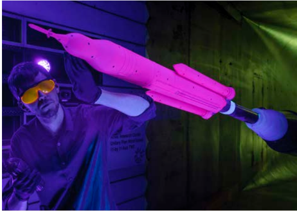
Dr. Patrick Shea inspects a 1.3 percent scale model of the second generation of NASA's Space Launch System in a wind tunnel for ascent testing at Ames Research Center
