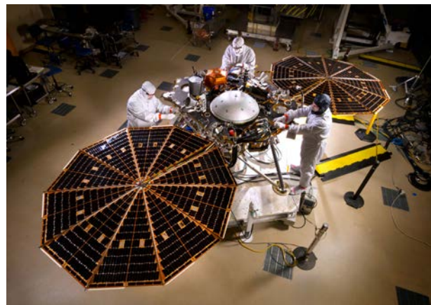
NASA's InSight Mars lander spacecraft deployed its solar arrays in a Lockheed Martin clean room near Denver
