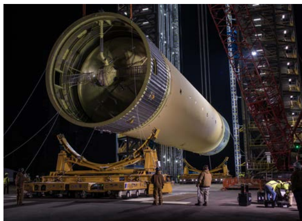
The SLS's liquid hydrogen tank test article is positioned in the test stand at NASA's Marshall Space Flight Center
