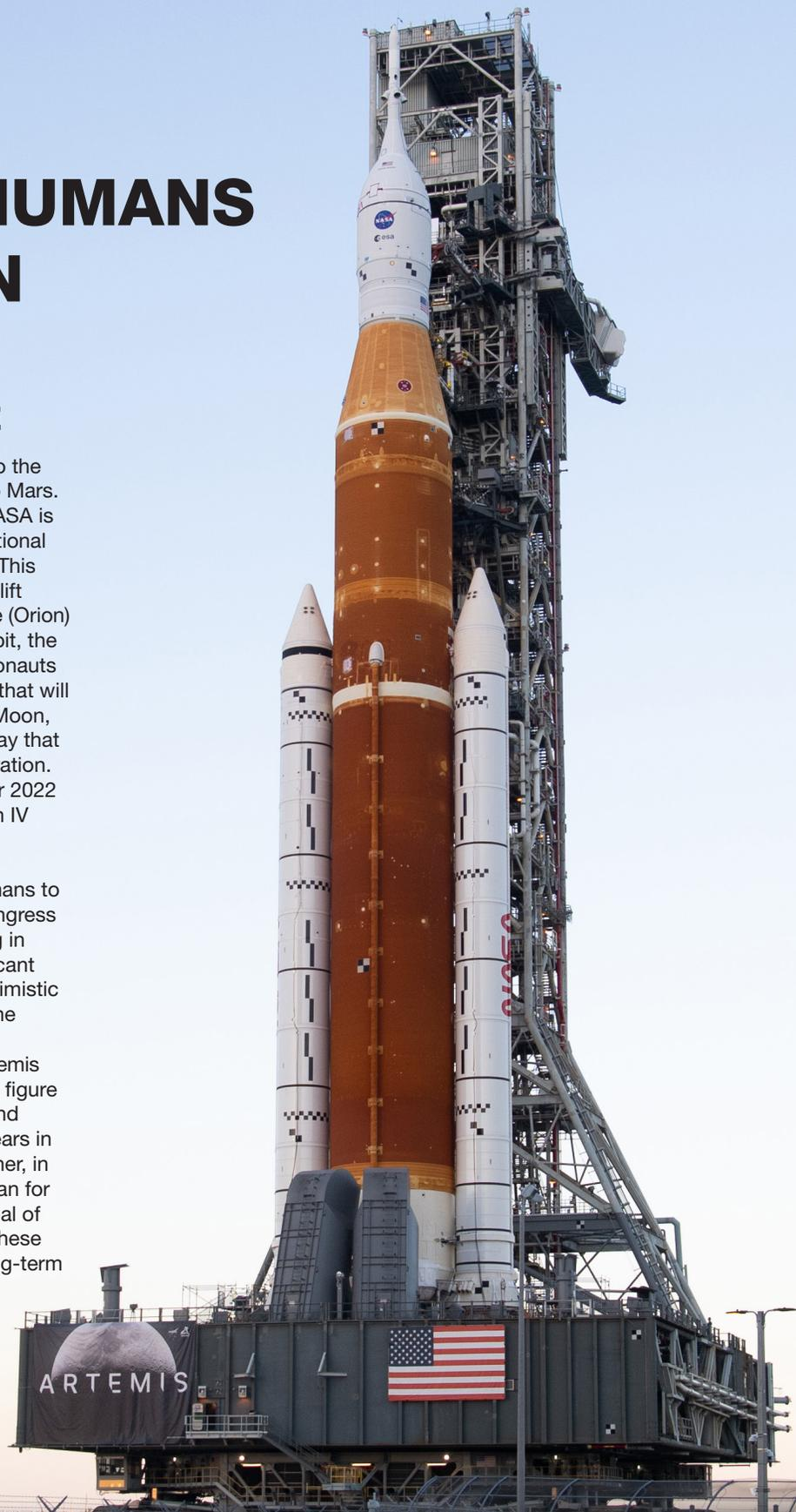
SLS rocket and Orion spacecraft atop a mobile launcher at Kennedy Space Center. Source: NASA
