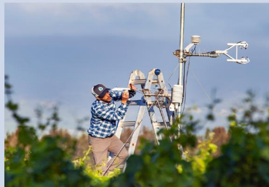
A research scientist with the NASA Ames Cooperative for Research in Earth Science and Technology adjusts a scientific instrument designed to support evapotranspiration data collection.
