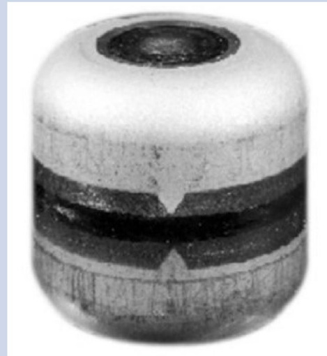
Pu-238 Pellet in its Protective Iridium Cladding
