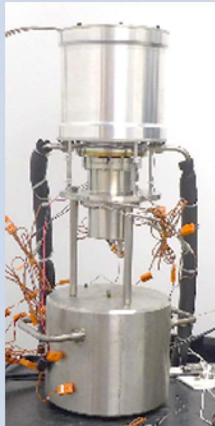
The Sunpower Robust Stirling Convertor prototype is being developed by Sunpower, Inc., of Athens, Ohio. The prototype is based on the Advanced Stirling Convertor from the ASRG flight development project.
