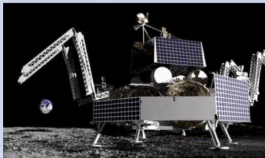
Illustration of the Griffin Lander on the Moon Deploying a Ramp for the Rover
