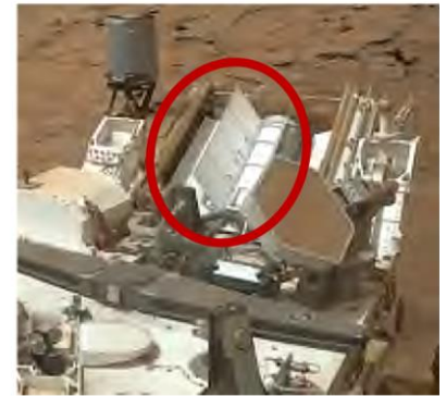
Image of the Mars Science Laboratory on Mars with the MMRTG structure (white object circled in red) visible.
