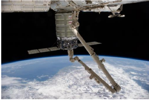
Orbital ATK Cygnus cargo vehicle docking at the International Space Station. Source: NASA.
