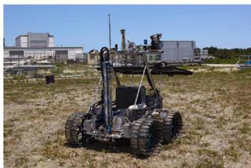
Regolith and Environment Science and Oxygen and Lunar Volatiles Extraction Rover. Source: NASA.
