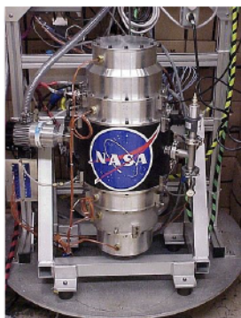
NASA G2 flywheel module used to store rotational energy for use by spacecraft. Source: NASA.
