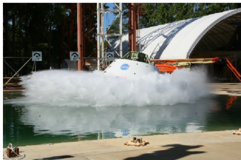
Orion drop testing at Langley. Source: NASA.
