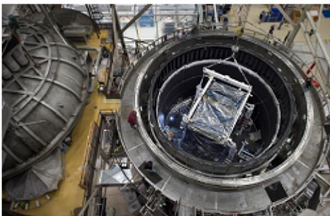
James Webb Space Telescope component undergoing thermal vacuum testing at Goddard. Source: NASA.
