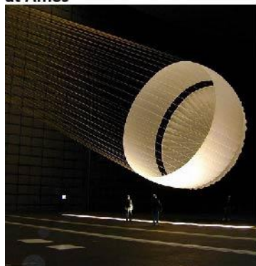
Mars Exploration Rover Parachute Deployment Testing at Ames
