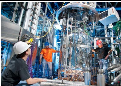
Workers at Glenn Research Center testing methods to reduce liquid hydrogen boil-off. Source: NASA.
