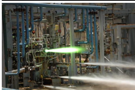
Testing of 3-D printed rocket with new copper alloys. Source: NASA.
