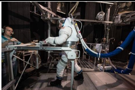
Human-in-the-loop testing of Portable Life Support System for an advanced space suit. Source: NASA.
