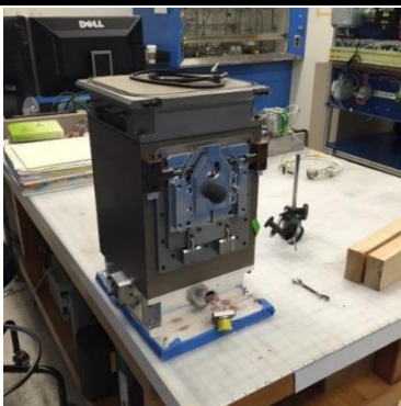
Heat Melt Compactor prototype to consume waste on the International Space Station. Source: NASA.
