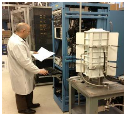
Advanced stirling convertor, white box on right, being tested at Glenn Research Center. Source: NASA.
