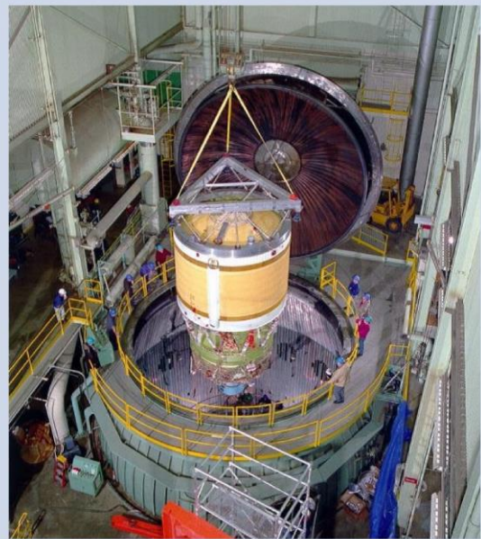
Delta III Rocket Components Being Lowered into the B-2 Thermal Vacuum Chamber
