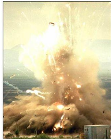
Figure 4. Destructive test of solid rocket motor
