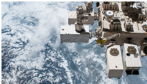
The Ecosystem Spaceborne Thermal Radiometer Experiment on Space Station experiment uses a radiometer mounted on the International Space Station to measure the temperature of plants on Earth. The project uses AI to automatically select and schedule scientific observations.
