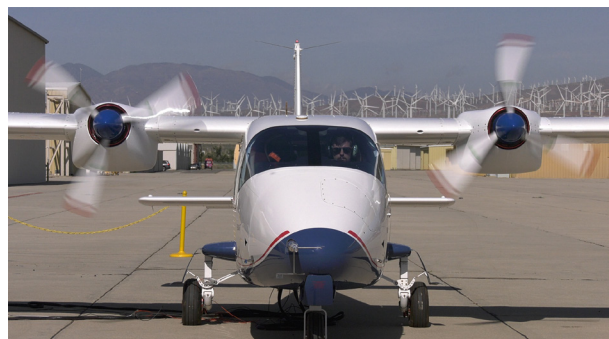
The electric motors for the X-57's Mod II vehicle and their propellers were powered up and spun together for the first time as part of an integrated spin test.
