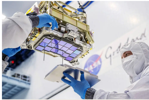
A technician at Goddard Space Flight Center installs a cover plate over the detectors for the Nancy Grace Roman Space Telescope. Each of the 18 detectors represents 16.8 million pixels of image resolution.
