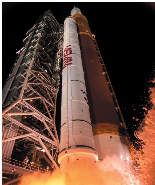
One of the Space Launch System's two solid rocket boosters fired up at liftoff during the Artemis I launch on November 16, 2022.
