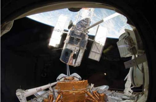
Space Shuttle Atlantis' robotic arm lifts the refurbished Hubble Space Telescope from the Shuttle's cargo bay on May 19, 2009. Source: NASA
