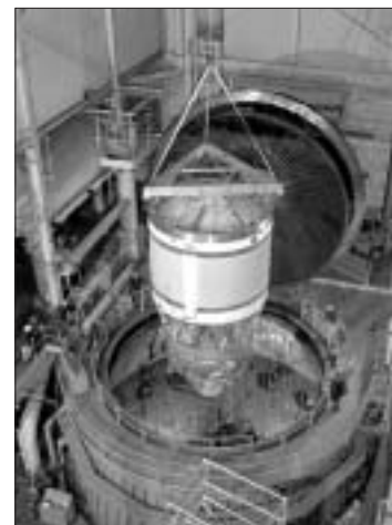
Stage of Delta III rocket being lowered into a test chamber at Plum Brook.
