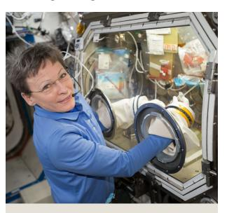
Microgravity Science Glovebox inside the ISS National Laboratory
