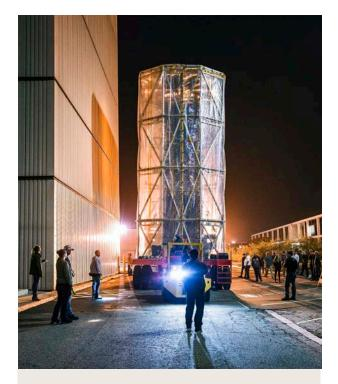
The James Webb Space Telescope is enclosed in a protective clamshell that serves as a mobile clean room while in transport.
