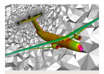
This image shows the aerodynamic properties of NASA's Transonic Truss-Braced Wing concept: red and violet show areas of higher drag, while green and blue show areas of lower drag. The geometric formations represent airflow around the aircraft, helping scientists understand the vehicle's aerodynamics and improve its efficiency.
