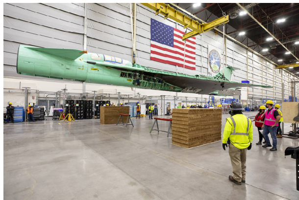
NASA’s X-59 Quiet SuperSonic Technology aircraft is prepared for the installation of the landing gear and other hardware required for structural testing. Image credit: Lockheed Martin
