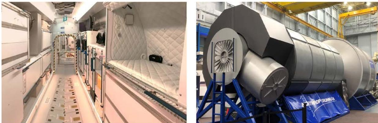
*Northrop's habitat prototype developed during NextSTEP-2, with an interior view to the left and exterior view to the right.*
