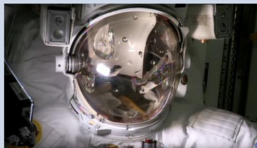
Recreation of Water Intrusion Incident Experienced During EVA 23
