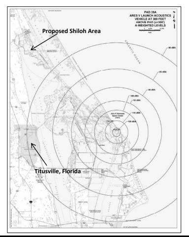
Source: NASA's Final Constellation Programmatic Environmental Impact Statement, January 2008, "Weighted Maximum Sound Pressure Level Contours for an Ares V Launch." NASA Office of Inspector General added the location captions.
