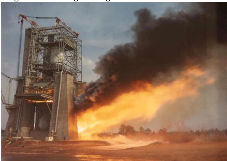
Figure 4. First Stage Testing of the Saturn V Launch Vehicle
